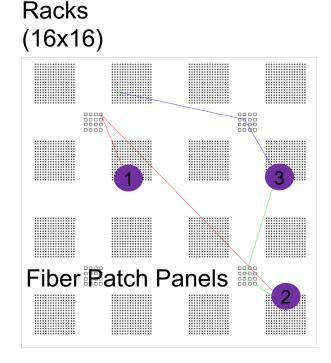
Small network with Mesh U/ECMP example (i.e. Unequal Multi-Path)
