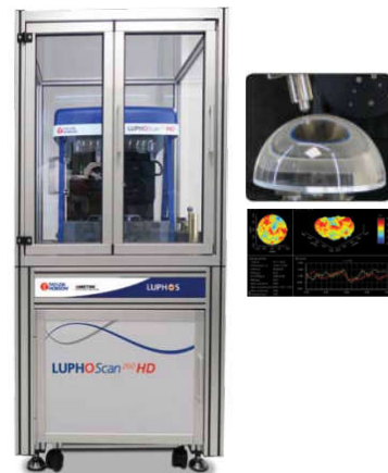
Taylor Hobson LuphoScan 260 for irregularity measurement Measure range: from 5 to 260 mm High surface accuracy: \pm 50\text{nm}
