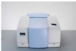
Spectrum 100FTIR for 2500-20000nm spectral region
