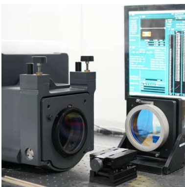
ZYGO Interferometer for high accuracy measurement of wave front & flatness & parallelism With \lambda/50 accuracy
