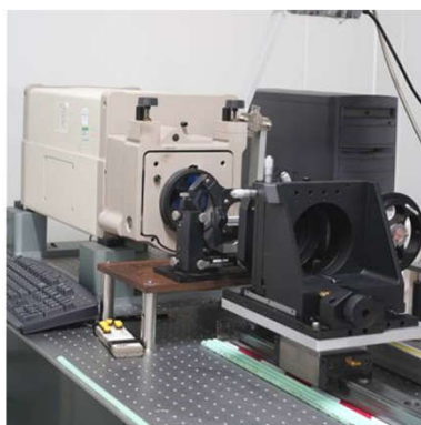
ZYGO Interferometer for high accuracy cylindrical surface measurement CGH transmission spheres: \lambda/10 surface accuracy
