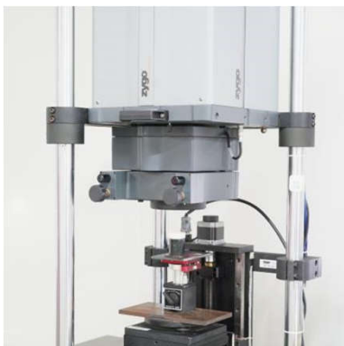
ZYGO GPI-XP Interferometer measure power & irregularity(P-V) with \lambda/50 accuracy
