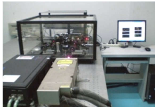
Bulk and surface absorption testing by PCI (355nm,532nm,1064nm)
