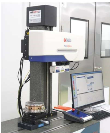
Taylor Hobson Form Talysurf PGI Measure range: from 0.1 to 200 mm Resolution ratio: 0.8nm
