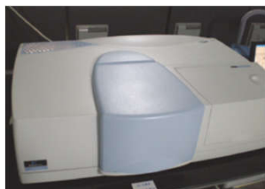
Perkin Elmer Lambda-950 for 175-3300nm spectral region
