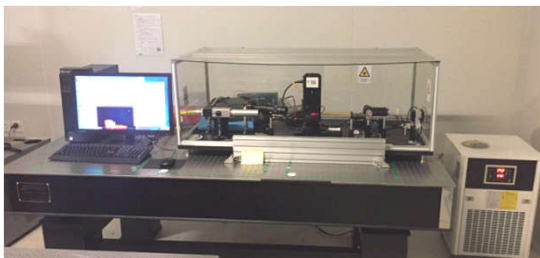
1064nm laser damage threshold testing system(CW,100W)
