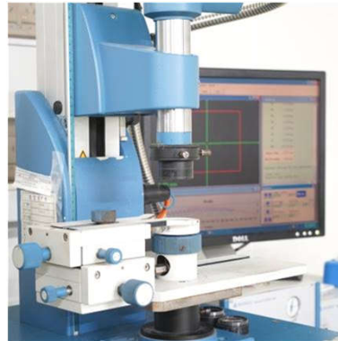
Trioptics OptiSpheric for comprehensive testing of optomechanical parameters of lenses
