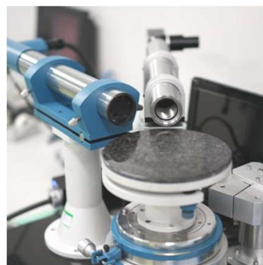
Trioptics PrismMaster for high-precision optical angle measurement with angular accuracy: 0.75''
