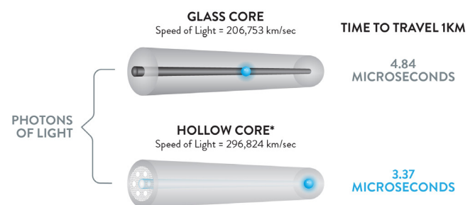
FIGURE 5: The speed advantage of light through a hollow-core fiber compared to glass fiber is 1.5 microseconds per km
