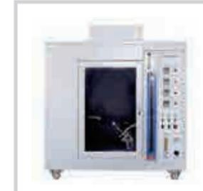
HORIZONTAL-VERTICAL BURNING FLAME TEST
