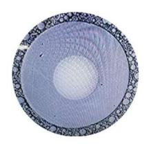
MPO/MTP CO Polishing Slurry surface after polishing: (400X Fiber-End Inspector)
