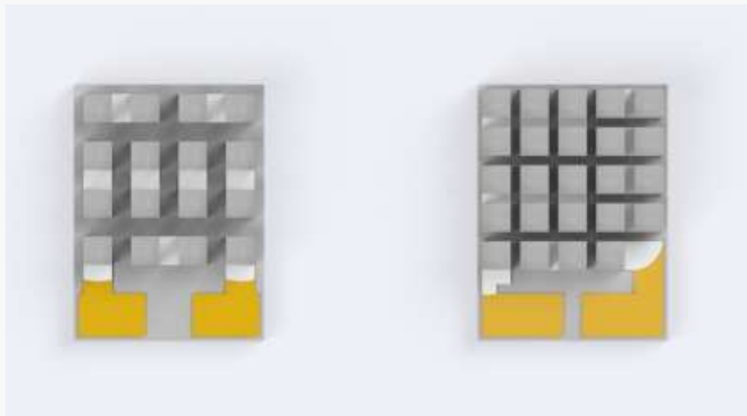
Fig.1 – Pellet density comparison of 1MD03-008-XX TEC and 1MDD03-012-XX TEC of the same size
