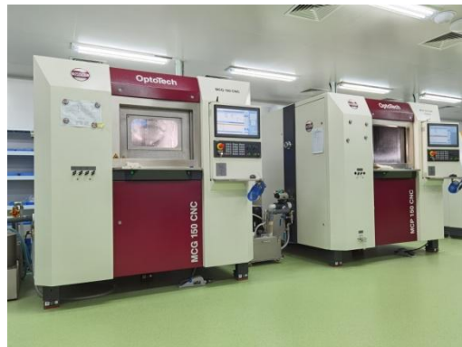
Aspherical CNC machining center
