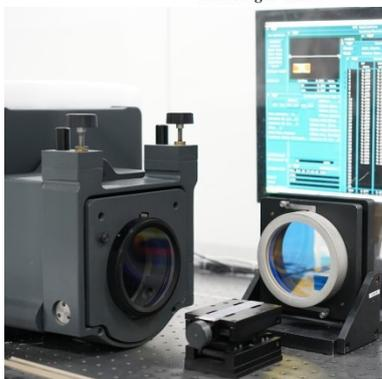
ZYGO Interferometer for wave front & parallelism Measurement
