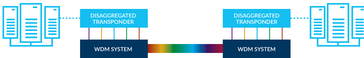
Figure 1 Datacenter interconnect optical solution (disaggregated solution)
