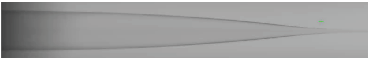
A Lensed Fiber being Drawn and Viewed using the FFS3 Software Suite, Included with Each Glass Processor
