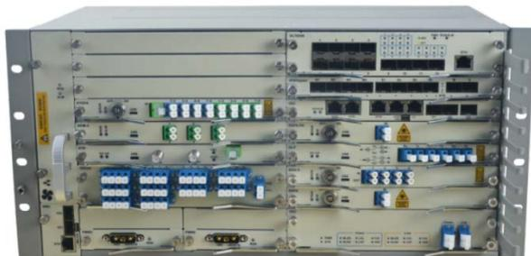
In response to the growing demand for higher capacity data streams in the DCI, after a period of system testing, B&A released the OTU400G service card based on the 400G-ZR optical transceiver(DCO) in February. Combined with the WSS-32 service card(Flex-Grid)
