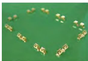
Shield-can clips reflow soldered onto PCB
