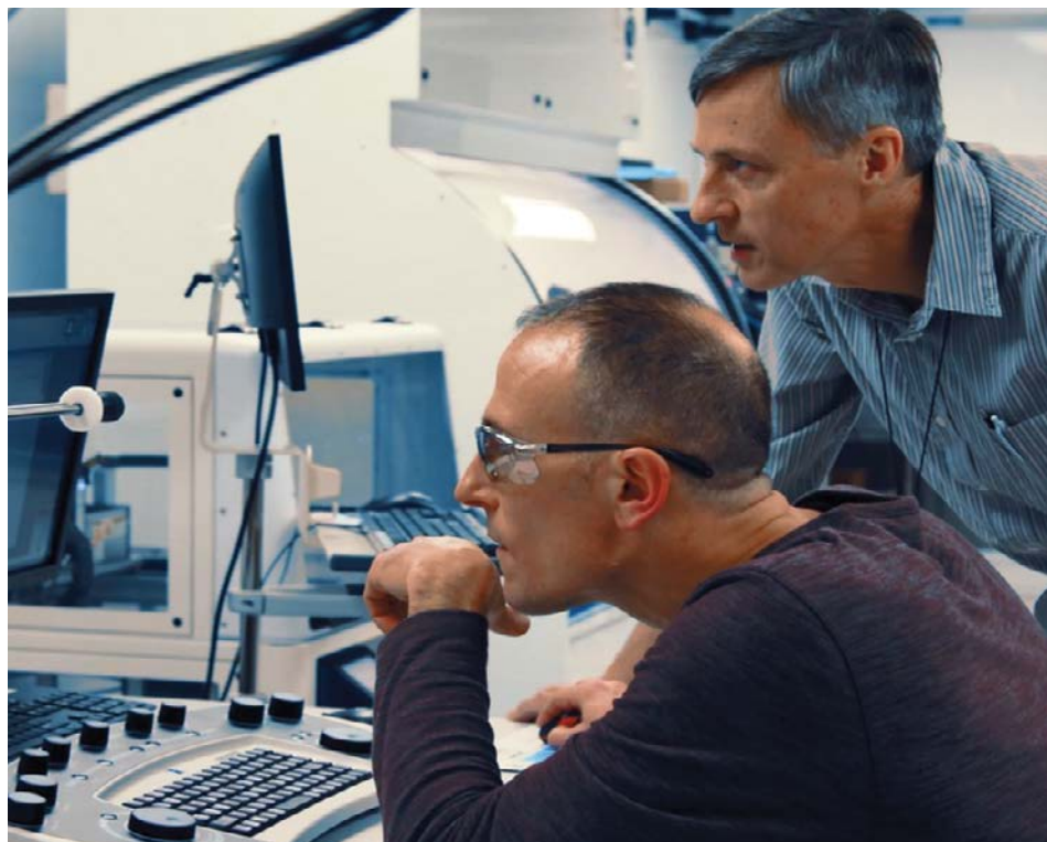
Engineers use an X-ray fluorescence tool to analyze wafers in AIM’s test, assembly and packaging (TAP) facility in Rochester, N.Y.
