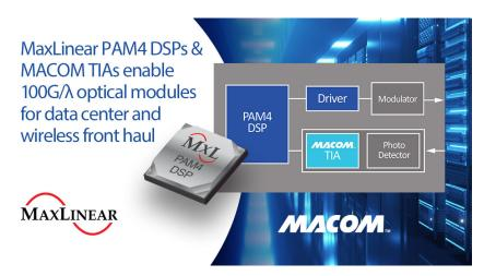
The collaboration includes pairing the MxL93516, MaxLinear's secondgeneration 100G Snowmass DSP, with MACOM's low power MATA-05817 100G TIA to achieve exceptional sensitivity and a low BER floor. This configuration is ideal for 100G-DR1/FR1/LR1 QSFP28 applications for Data Center and front haul applications.
