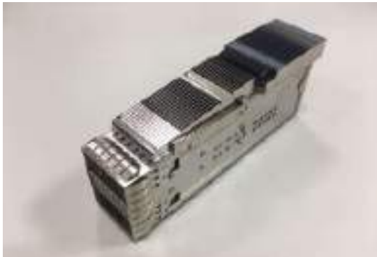
Figure 2-5: QSFP-DD stacked card cage
