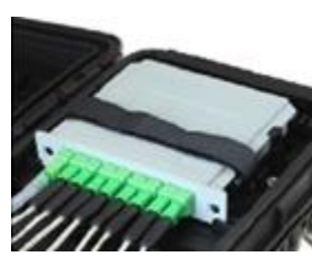
Top Layer: Splitter Ports for Drop Cable Connections
