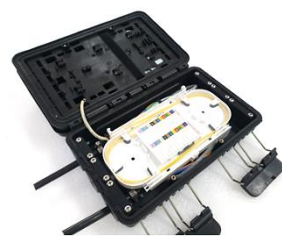
Middle Layer: Splice Tray for Feeder Fiber Integration
