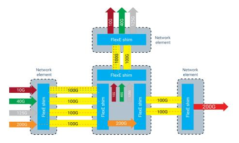
Figure 7. FlexE channelization example
