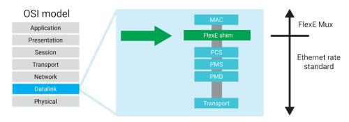
Figure 4. Characteristics of FlexE shim
