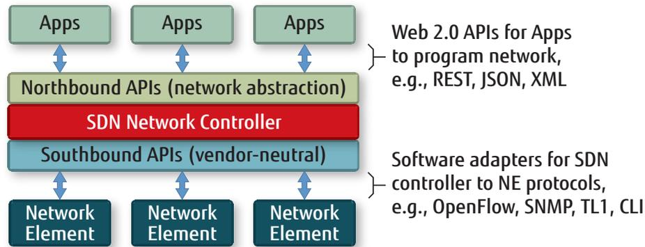
**Figure 1: SDN Basic Architecture**
