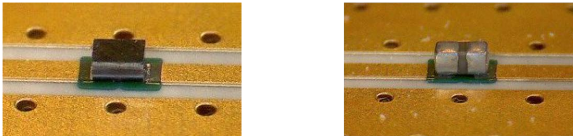
Figure 2: Silicon capacitor used as SMD compared with MLCC SMD
